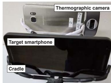
Figure 1: Measurement setup.
