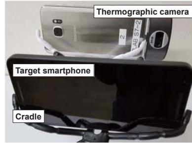
Figure 1: Measurement setup.
